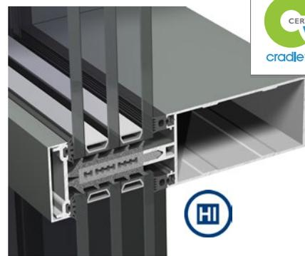
VARIANTE CW 50 POSE EN RUBAN (STRUCTURE PRÉASSEMBLÉE)
